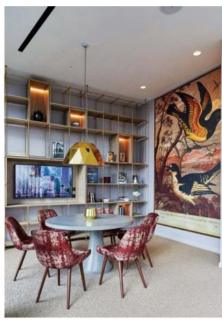
Hundreds of brass tubes were fitted together using intricate brackets to form these floor to ceiling display shelves.
